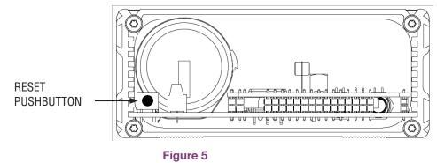
While pressing and holding the reset button, place the power switch in the ON position. After 5 seconds, the STATUS LED will light for a full 3 seconds indicating that the default settings have been initiated. Release the reset button and turn the unit power switch OFF. When the unit is powered again, the unit will have the default settings restored. Note that this second power cycling following the reset is necessary to fully load the reset parameters.
